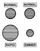
The largest pan which you should use on any burner is 230mm (9"). The base of the smallest pan should not measure less than 100mm (4").
